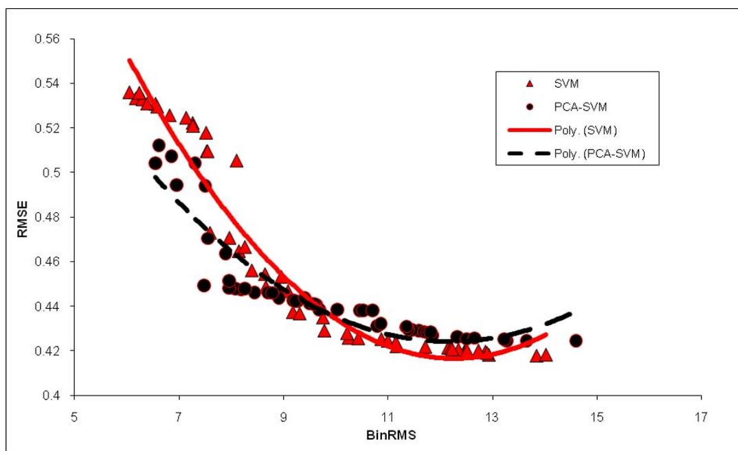
Figure 3: Trade-off curve between the two objectives BinRMS vs. RMSE for SVM and PCA-SVM
