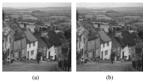
Fig. 9. The decrypted image when encrypted image is disturbed by SPN attack. (a) The density of SPN is 10^{-3} . (b) The density of SPN is 10^{-2} .
