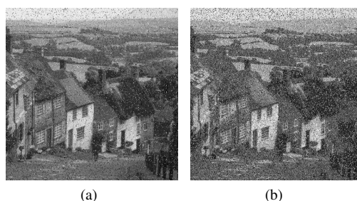
Fig. 11. The decrypted image when encrypted image is disturbed by SN attack. (a) The variance of SN is 10^{-3} . (b) The variance of SN is 10^{-2} .
