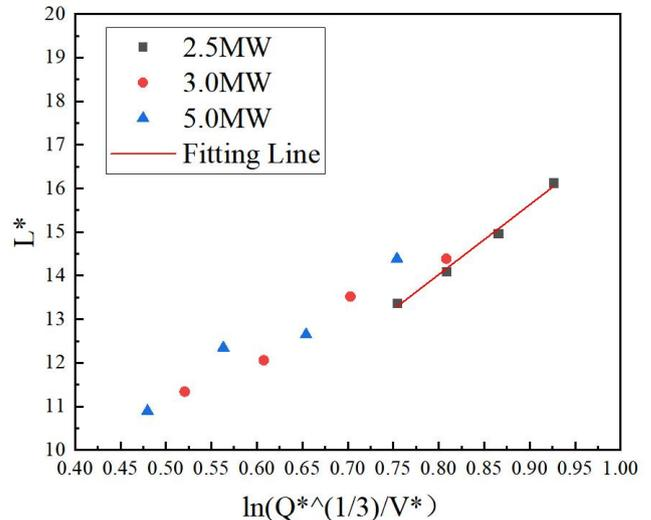
Fig. 6. Correlation of dimensionless smoke counterflow length with variable of  $\ln(Q^{*(1/3)} / V^*)$  with high HRR.
