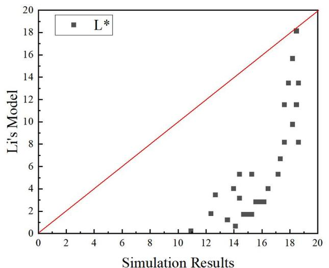
Fig. 7. Comparison between simulation results and Li model prediction of smoke counterflow length
