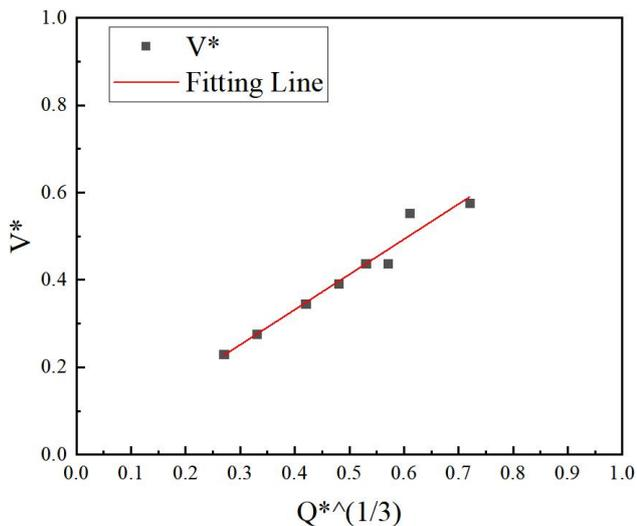
Fig. 4. The dimensionless critical ventilation speed in the tunnel.
