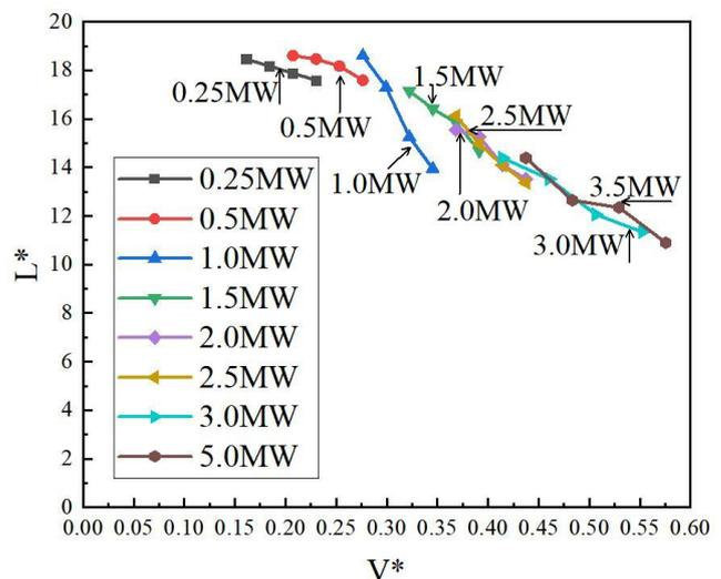
Fig. 3. The dimensionless smoke counterflow length in the tunnel with dimensionless ventilation speed.
