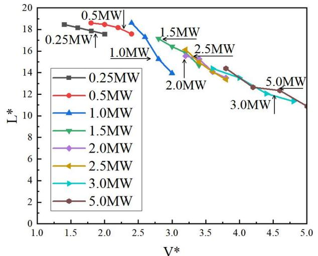
Fig. 2. The smoke counterflow length in the tunnel with ventilation speed.
