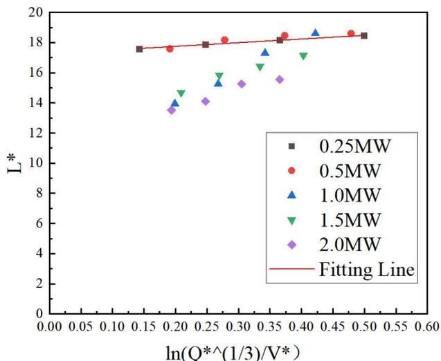
Fig. 5 Correlation of dimensionless smoke counterflow length with variable of  $\ln(Q^{*(1/3)} / V^*)$  with small HRR.
