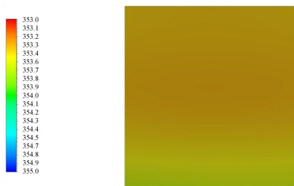
Fig. 4 Distribution of water molar concentration in PEMFC
