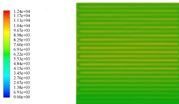
Fig. 3 Distribution of current density in PEMFC
