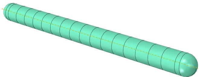
Fig. 5. Pressure-resistant shell finite element model
