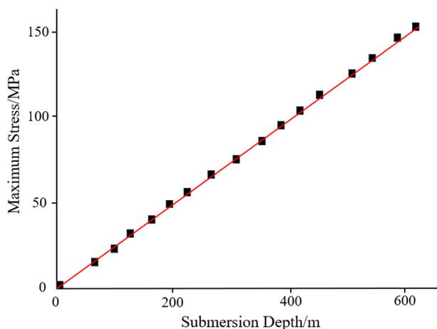
Fig. 7. Fitting curve of diving depth and maximum stress
