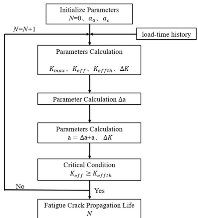
Fig. 4. Numerical integration method by cycle
