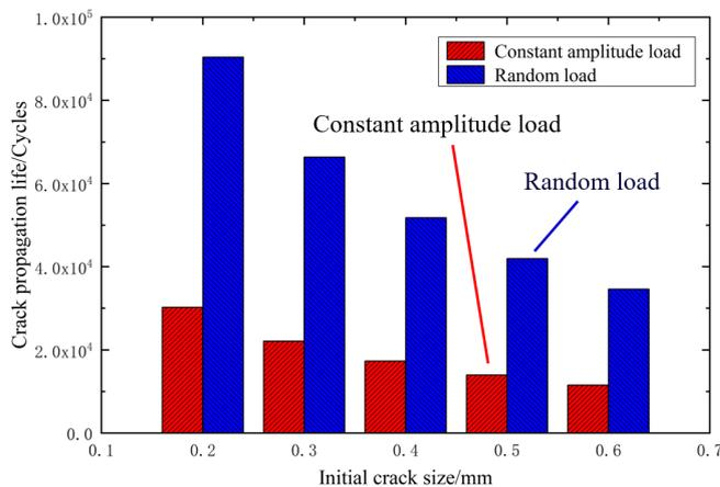
Fig. 8. Fatigue life of different initial crack depths
