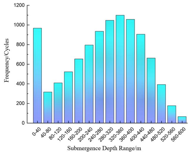
Fig. 2. Fatigue load spectrum of 600m deep underwater vehicle
