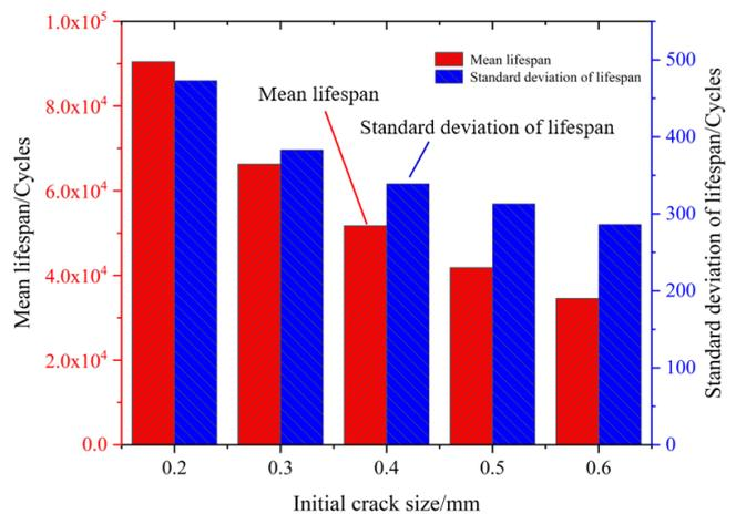
Fig. 10. The mean value and standard deviation of fatigue life under different initial crack sizes
