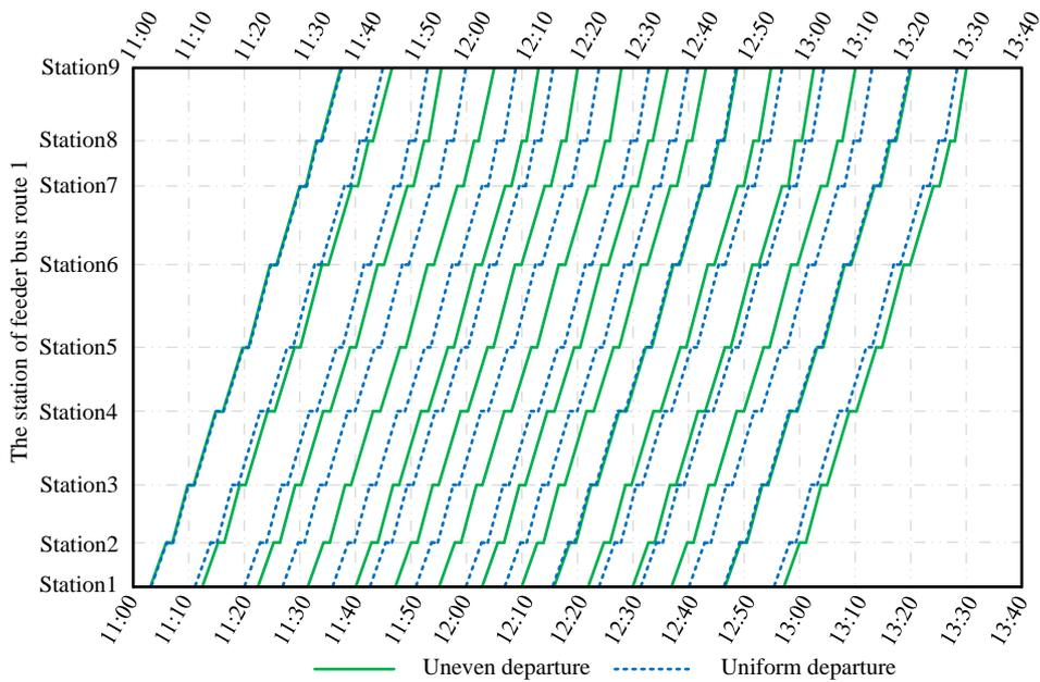
Fig. 12. Bus operation diagram of different departure modes (The feeder bus route 1)
