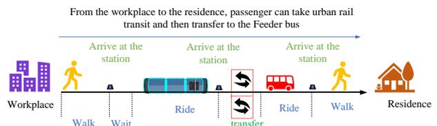
Fig. 2. The integrated transfer process of urban rail transit and feeder bus
