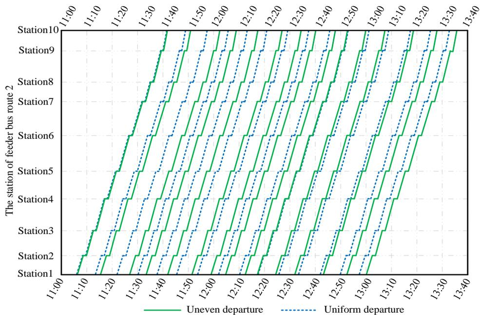
Fig. 13. Bus operation diagram of different departure modes (The feeder bus route 2)
