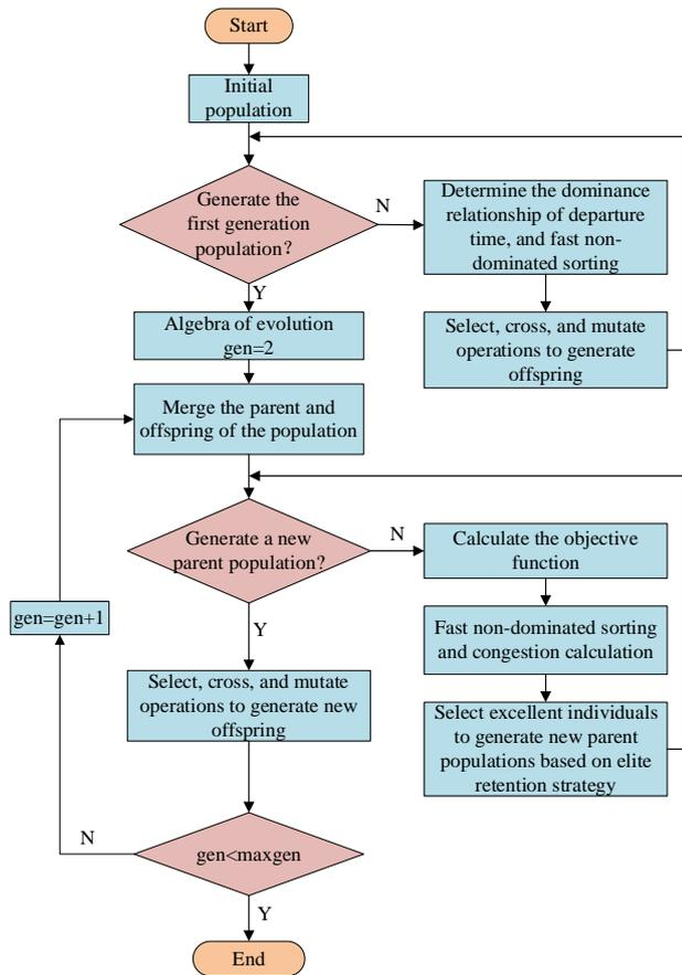
Fig. 8. NSGA-II algorithm flowchart
