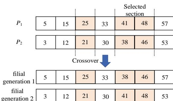
Fig. 6. Schematic diagram of Crossover operation
