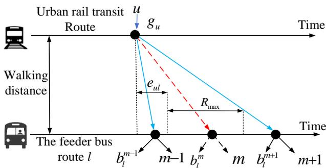
Fig. 3. Time and space diagram of transfer between urban rail transit and feeder buses
