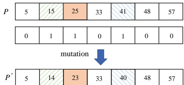
Fig. 7. Schematic diagram of mutation operation
