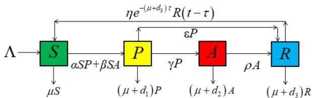
Fig.1. Transfer diagram of the SPARS model with time delay.
