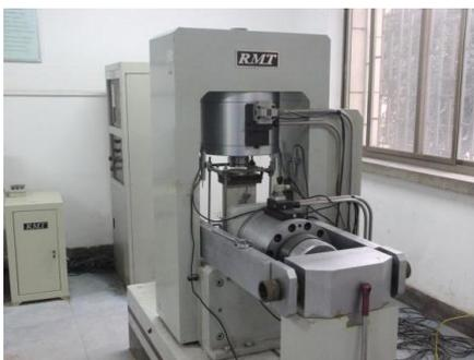
(a) RMT-150B rock mechanics test equipment
