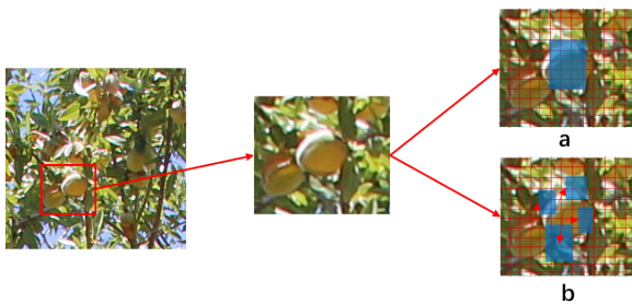
Fig. 8: Convolution process of conventional convolution (a) and DCNv2(b)
