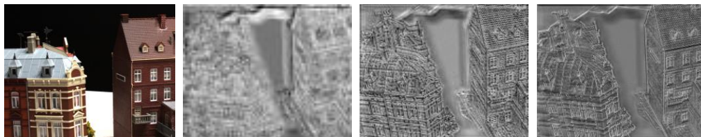
Fig. 5. Plots of Laplace pyramid residuals at different scales, from left to right, original, residuals with 8-fold down-sampling, residuals with 4-fold down-sampling, residuals with 2-fold down-sampling
