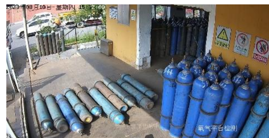
Fig. 2. Oxygen cylinder rolling on the ground
