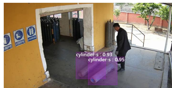
Fig. 7. Detection of fallen oxygen cylinders
