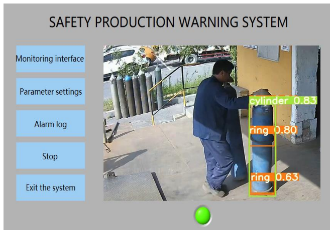
Fig. 14. Safety production warning system
