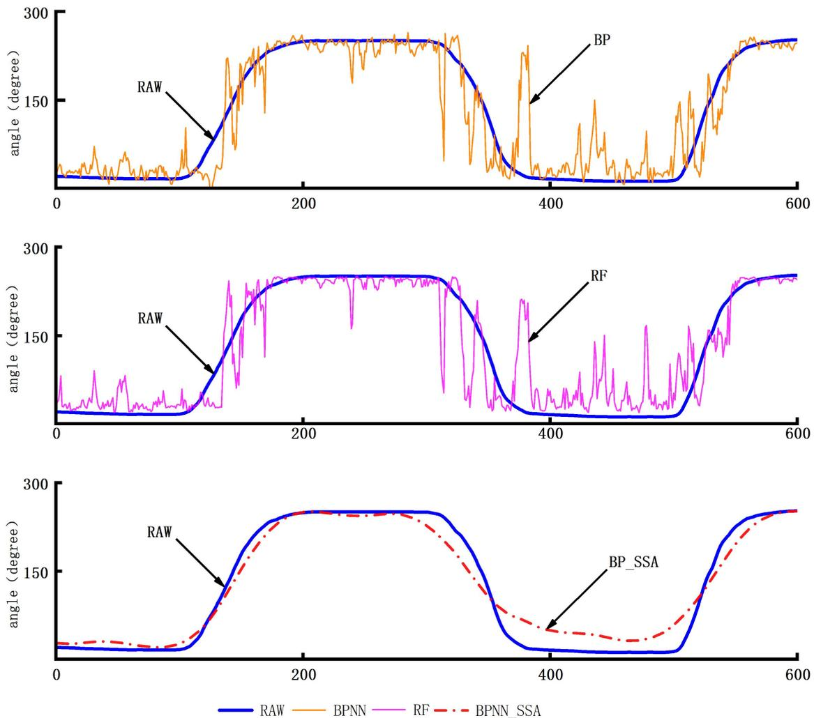
Figure 7. Comparison of Four-Finger Joint Angles at the Finger Extensor Area Between Different Models.
