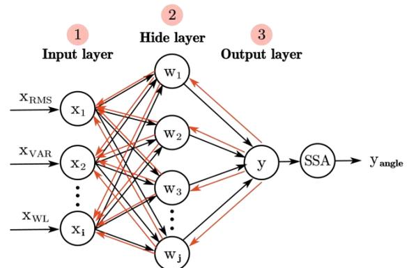
Figure 3. Schematic diagram of the BPNN\_SSA algorithm.
