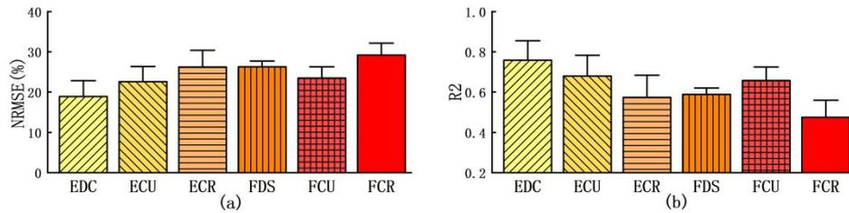
Figure 5. Compares the estimation accuracy of sEMG signals across six channels. (a) NRMSE values, (b) R<sup>2</sup> values. Bar graphs represent means, and error bars are the standard error of the mean.
