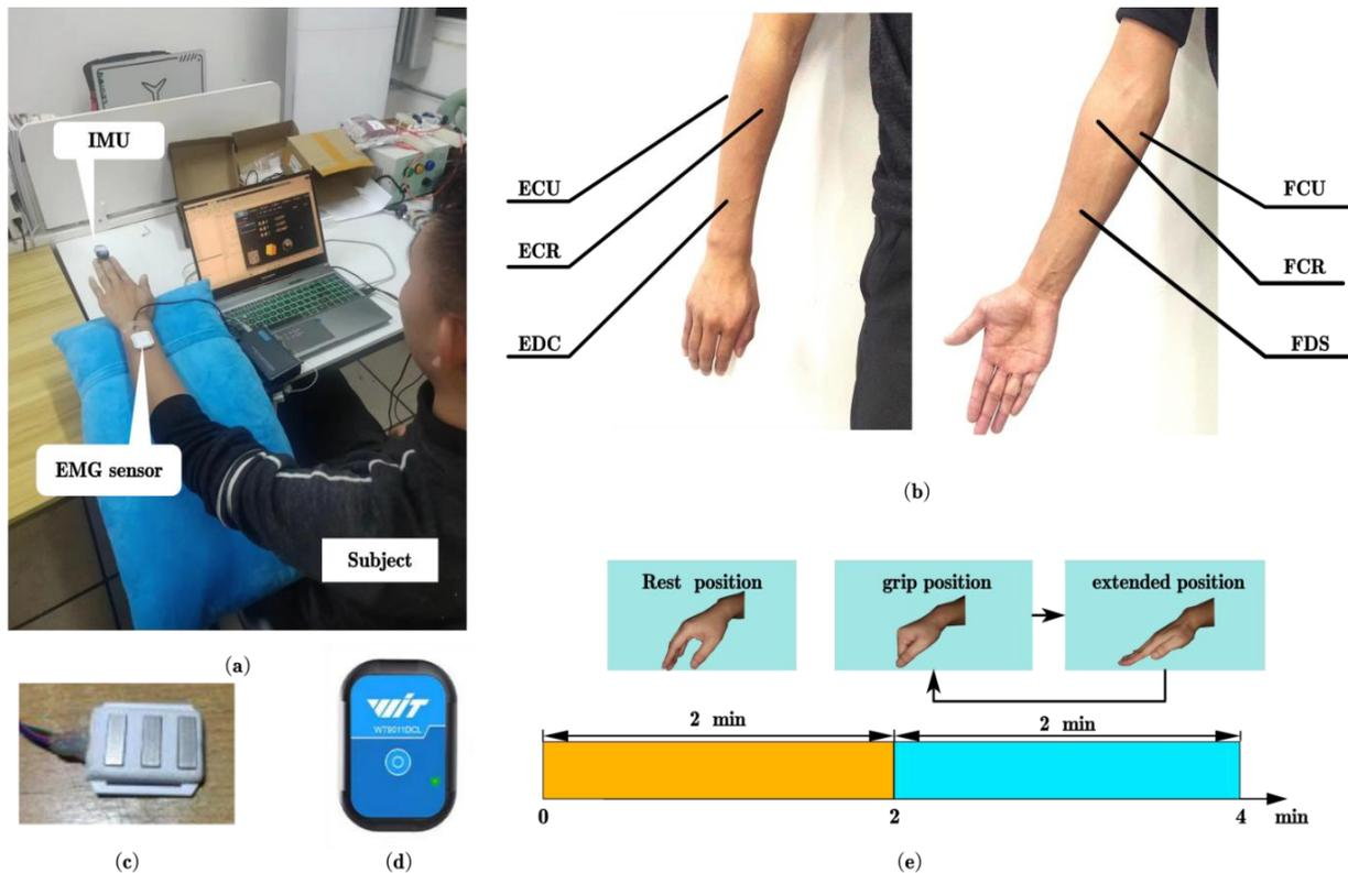
Figure 2. Experimental Setup: (a) Schematic diagram of experimental data collection, (b) Placement of electrodes for EMG signal acquisition, (c) EMG sensors, (d) IMU, (e) Time and sequence of actions performed by the user in a single trial.
