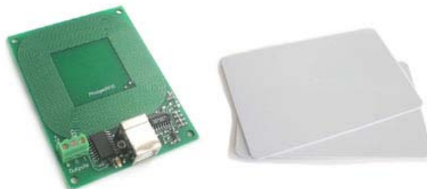
Fig. 3 RFID reader and cards within tag
