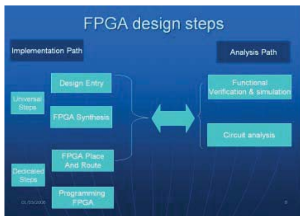
Figure 3: FPGA Design Steps
