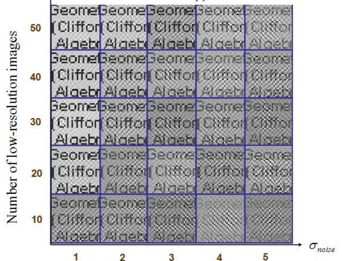
Figure 4 : Reconstructed super-resolution images using the MLE
