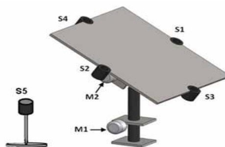
Figure 2. Solar tracker sensors
