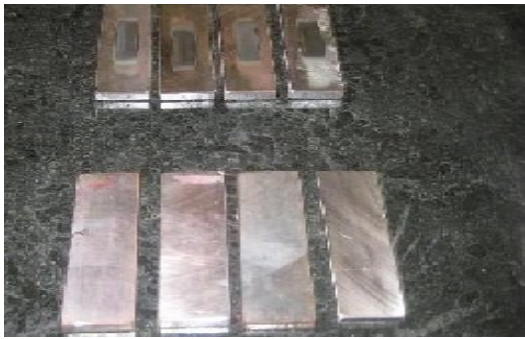
Figure 1: Standard Test Specimen (75x26x6 mm)
