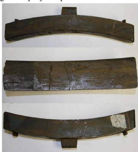
Fig. 2: Used low friction brake blocks from a wagon company
