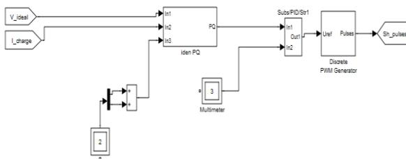
Fig. 2. Control of shunt active filter
