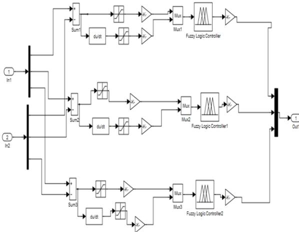
Fig.3. Fuzzy logic controller of Shunt active filter
