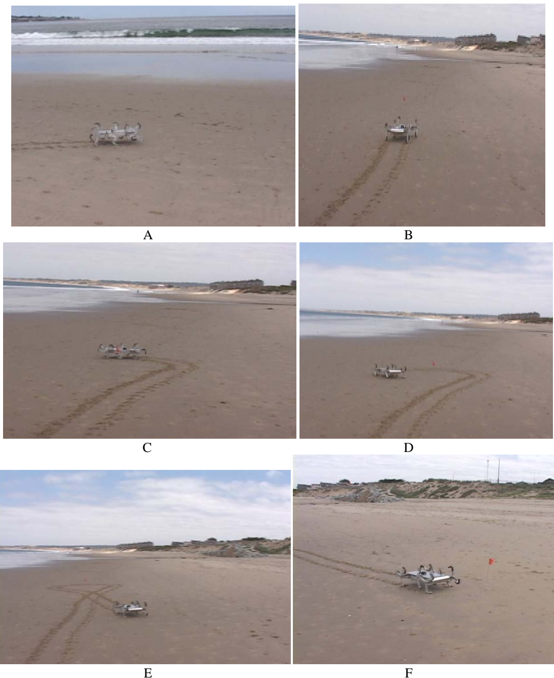
Figure 11 (a-f): Progressive snapshots of the robot walking autonomously on a beach in Monterey, CA to reach waypoints
