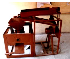
Fig. 1: The Palm kernel oil extractor
