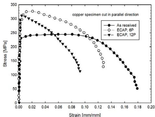
Figure 1: Stress-strain curves for the copper alloy samples cut in parallel direction
