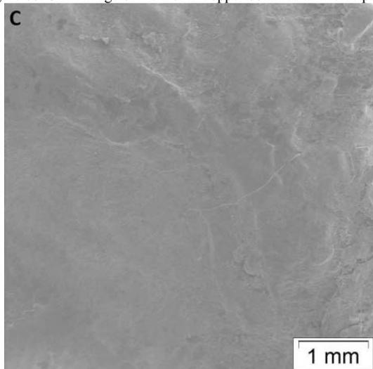
Figure 6c: SEM image of Fracture surface of processed UFG copper
