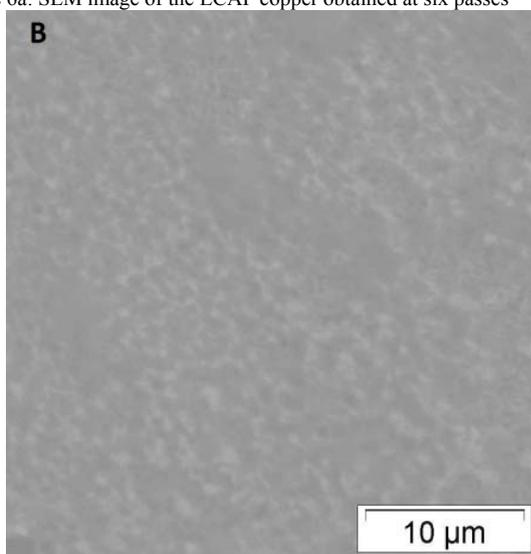
Figure 6b: SEM image of the ECAP copper obtained at twelve passes
